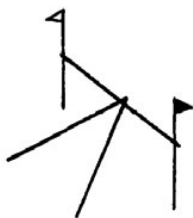
Neither end of sloping poles is supported by standard cup or fitting
